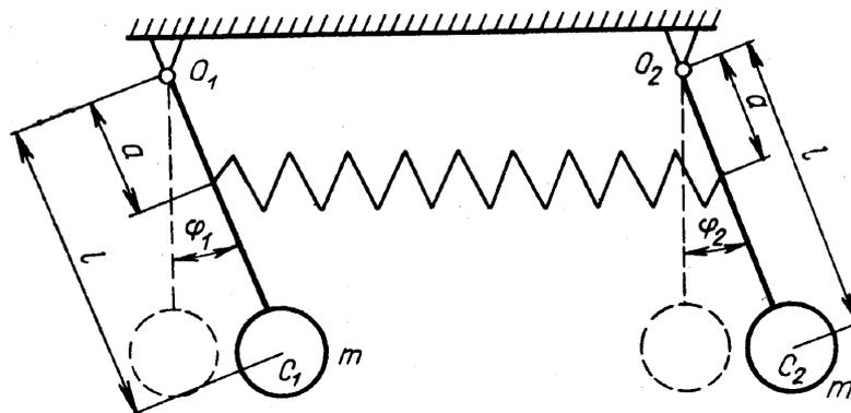
$$\begin{aligned} q_1 &= \varphi_1, \\ q_2 &= \varphi_2. \end{aligned}$$
