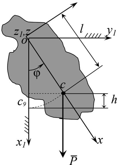
$$\begin{aligned} q &= \varphi, \quad T = \frac{1}{2} I_z \dot{\varphi}^2 \\ \Pi &= Ph = mgl(l - \cos\varphi) \\ I_z &= I_{z_c} + ml^2 \\ \cos\varphi &= 1 - \varphi^2 / 2 + \dots \\ \frac{\partial \Pi}{\partial \varphi} &= mgl \sin\varphi \\ I_z \ddot{\varphi} + mgl \sin\varphi &= 0 \end{aligned}$$
