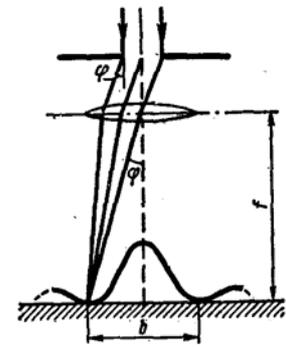
$$a \sin \varphi = \pm k\lambda, \quad k = 1, 2, 3, \dots \quad (2)$$
